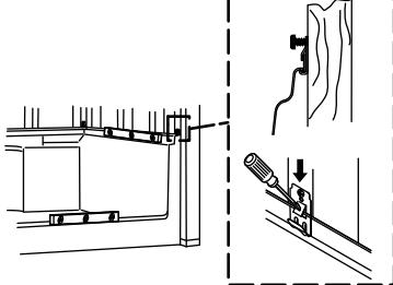
**9** Install plastic attachment clips at all remaining stud locations.
