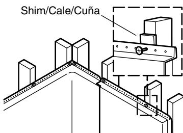
**19** Cover the framing with water-resistant wallboard. Install the finished wall material.
