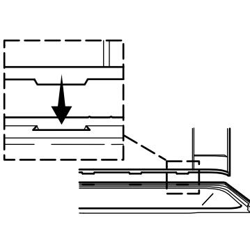
**14** Measure, mark, and drill the faucet holes in the drain end wall.
