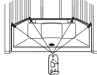
**8** Level the unit. Secure the metal support clips to the studs. Bend the tabs over the flange.
