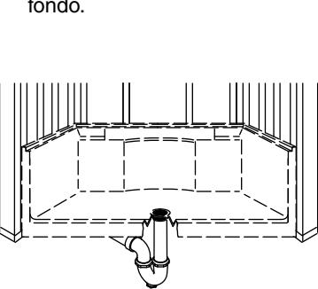
**12** To pre-fit the walls, remove the retaining clips. Reinstall the retaining clips before continuing.
