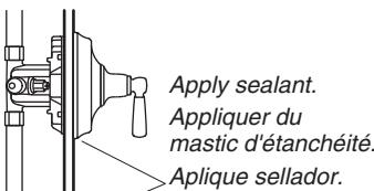
**21** After painting, apply 100% silicone sealant where the unit contacts the finished wall.
