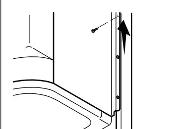
**18** Secure the walls to the studs along the top. Use shims as needed.
