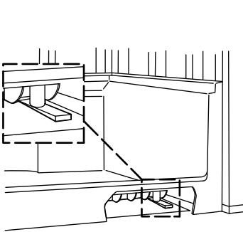
**11** Connect the drain to the drain pipe. Position a protective liner in the basin.
