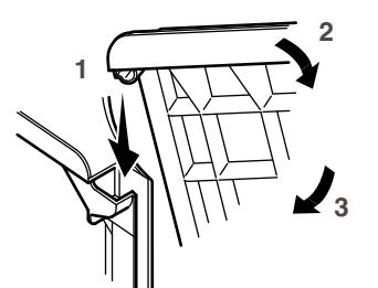
**16** The front edges should be flush, with no more than a 1/32" (1 mm) gap.
