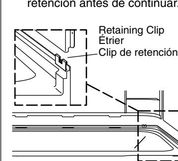
**13** Install the back wall. Insert the back wall tabs into the slots.
