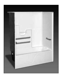
Specification – Oasis one-piece, 60 x 32-inch deep, FRP gelcoat bathtub model TS-6032, offered in a standard 16-inch or 17.25-inch (ABF) apron height. ActivLife package includes 2-horizontal bars on back wall along with a single horizontal bar on head end wall and on the control wall.
