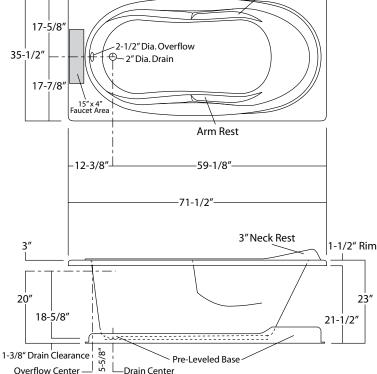
Sump Dimen: 54" long x 21" wide x 20-1/4" deep Sump Capacity: 78 gal. (unoccupied - to overflow) Whirlpool Operating: 53 gal.
