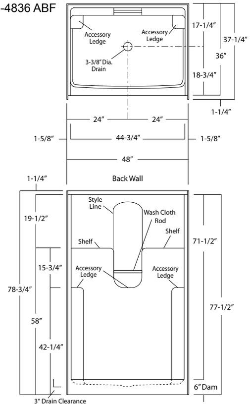
**Illustration 1b - Center Drain, Unit Dimension & Alcove Framing Guidelines (dimensional tolerance +0 / -3/8")**
