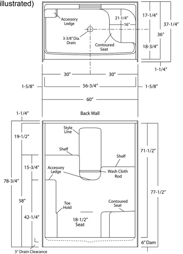
**Illustration 1c - Center Drain, Unit Dimension & Alcove Framing Guidelines (dimensional tolerance +0 / -3/8")**
