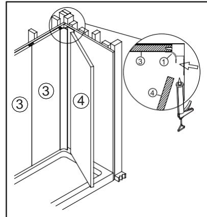
6. Press against the wall smoothing out any air bubbles along the entire area and then lightly tap on wall panel with a rubber mallet from top to bottom to ensure it is tightly connected to the wall.
