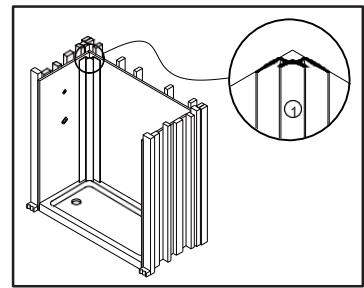
5. Peel off back of double-sided tape from the back of the panel. Position the panel at approximately 30 degrees, push the cut edge into the corner and then carefully push the panel towards the back wall.
