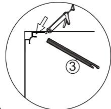
6. Push panel firmly against the wall smoothing out any air bubbles along the entire area and then lightly tap on wall panel with a rubber mallet from top to bottom to ensure it is tightly connected to the wall.
