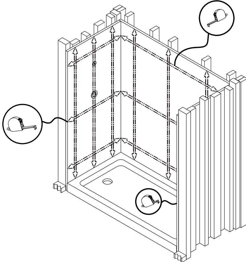
3. Measure cut-out locations for plumbing fixtures and mark them on the back of the appropriate panel(s).
