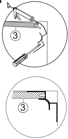
6. Press against the wall smoothing out any air bubbles along the entire area and then lightly tap on wall panel with a rubber mallet from top to bottom to ensure it is tightly connected to the wall.
