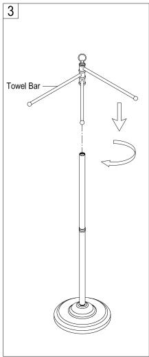
3. Install towel bar assembly onto rod by threading assembly in a clockwise direction.
