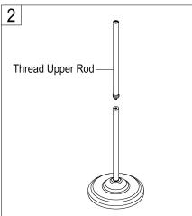
2. Thread upper rod onto lower rod, the end that has the decorative ring should be facing down.
