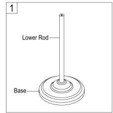
Place base on a flat level surface and thread lower rod onto base in a clockwise direction.
